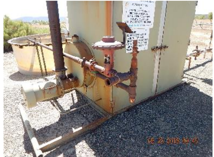
Photo 2: Separator with disconnected flow line.
