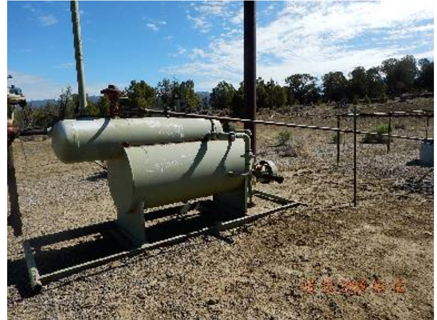
Photo 2: Separator with disconnected flow line.
