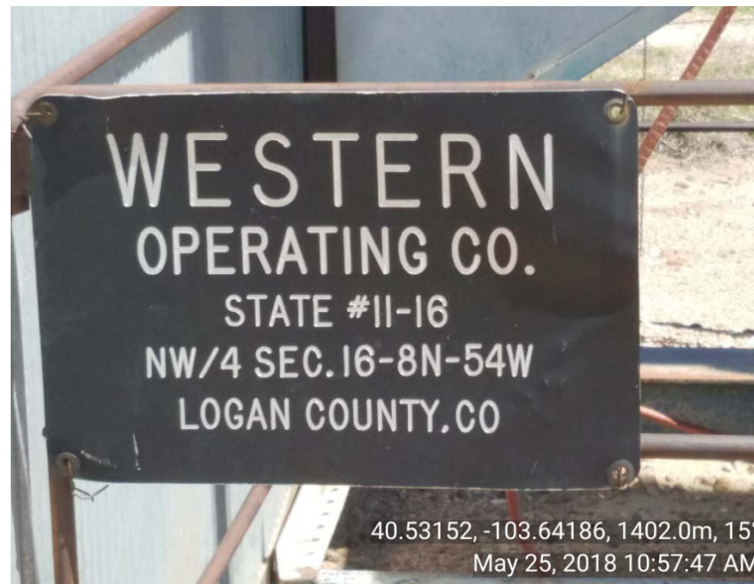
Photo 3: Incorrect sign at pump jack
