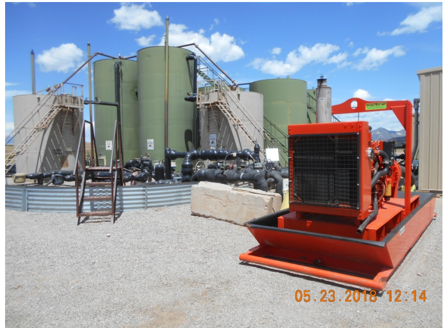
Tank battery and transfer pump
