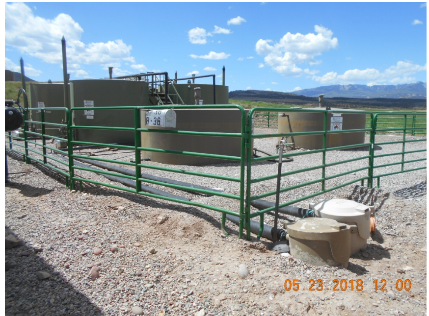
Production tank battery
