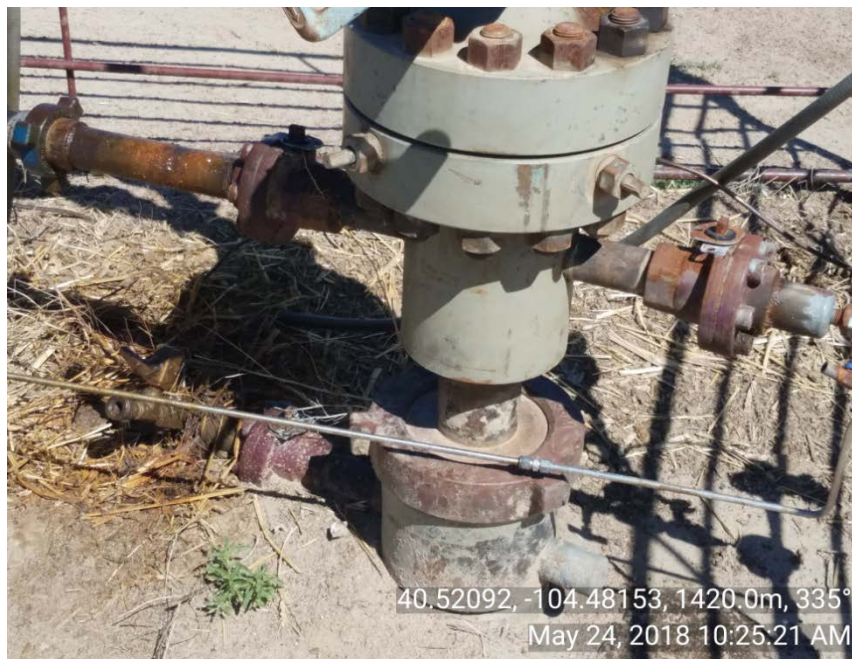
Photo 4: Stained soil at wellhead
