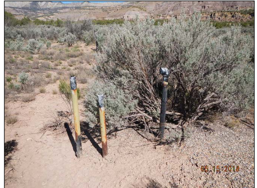
Photo 2. Disconnected flowlines.
