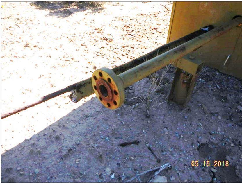
Photo 5. Meter run disconnected.
