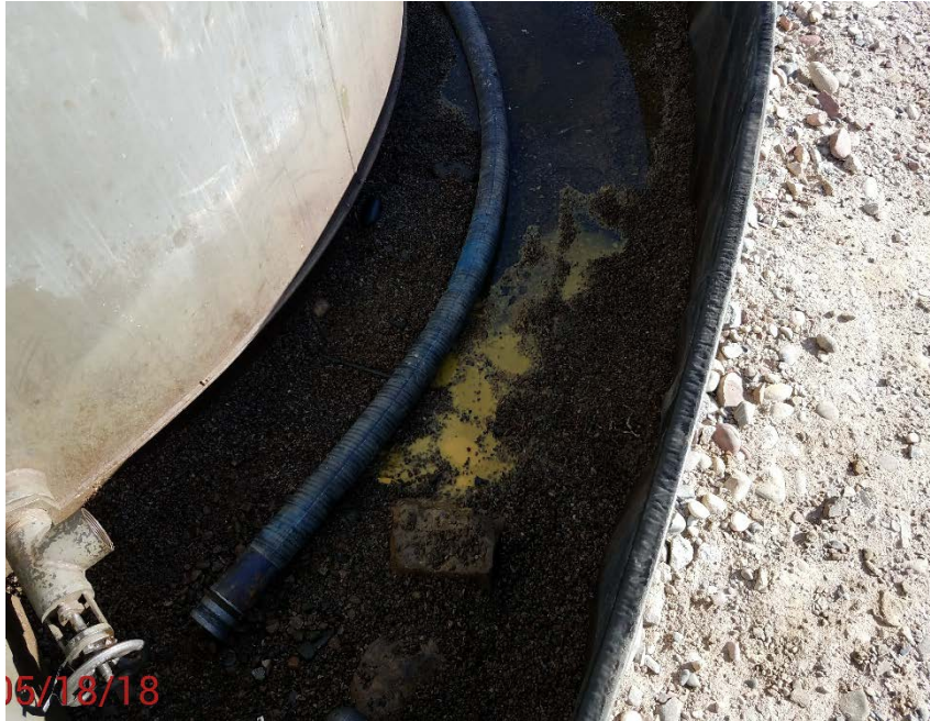
Location Photo #5, Condensate spilled in containment
