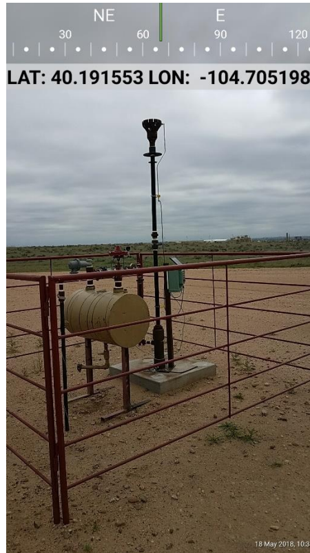
Photo 2 Bradenhead flare setup
