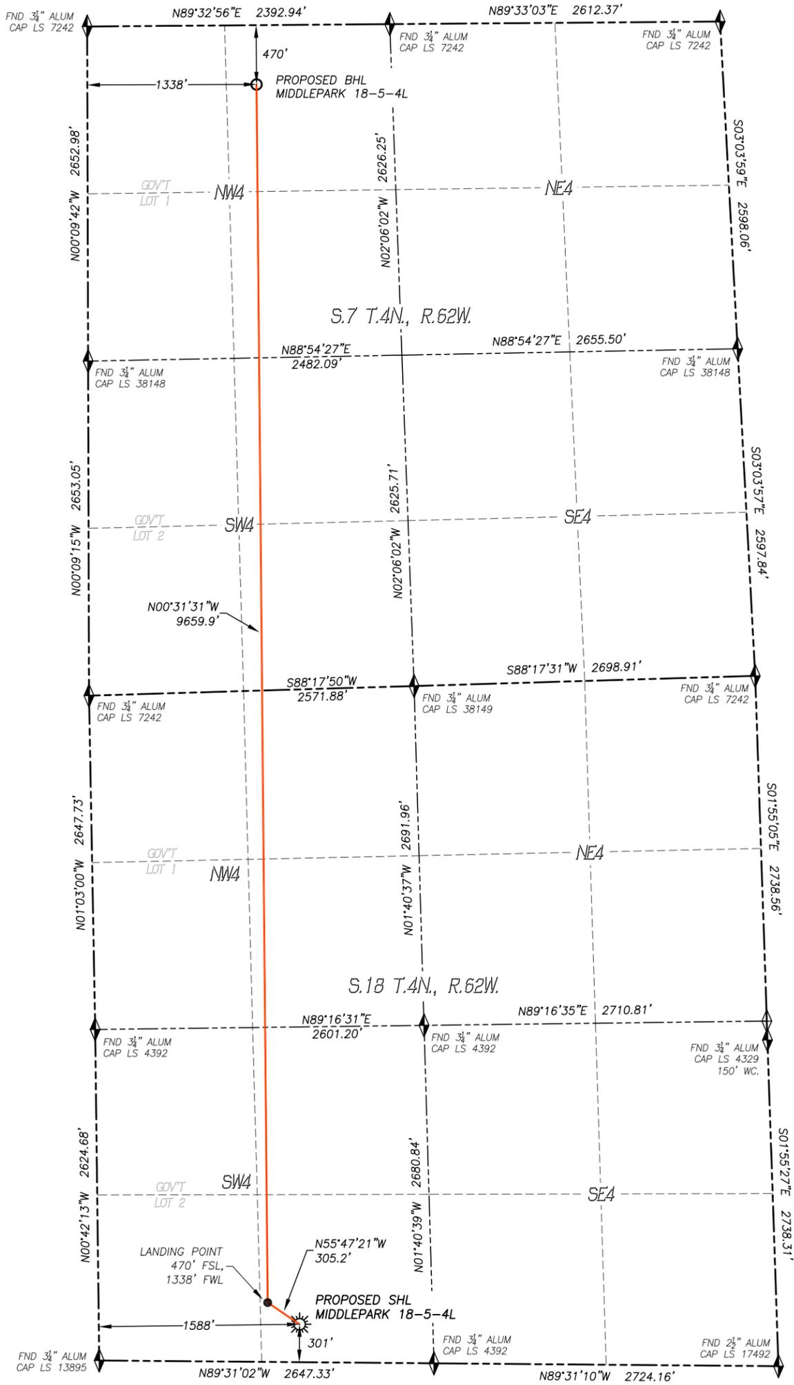
IN ACCORDANCE WITH A REQUEST FROM CONFLUENCE RESOURCES, DALEY LAND SURVEYING, INC. HAS DETERMINED THE SURFACE LOCATION OF THE MIDDLEPARK 18-5-4L WELL TO BE 301' FSL, 1588' FWL, AS MEASURED AT NINETY (90) DEGREES FROM THE SECTION LINES OF SECTION 18, TOWNSHIP 4 NORTH, RANGE 62 WEST, AND THE BOTTOM HOLE LOCATION TO BE 470' FNL, 1338' FWL, AS MEASURED AT NINETY (90) DEGREES FROM THE SECTION LINES OF SECTION 7, TOWNSHIP 4 NORTH, RANGE 62 WEST, OF THE 6TH PRINCIPAL MERIDIAN, WELD COUNTY, COLORADO.
