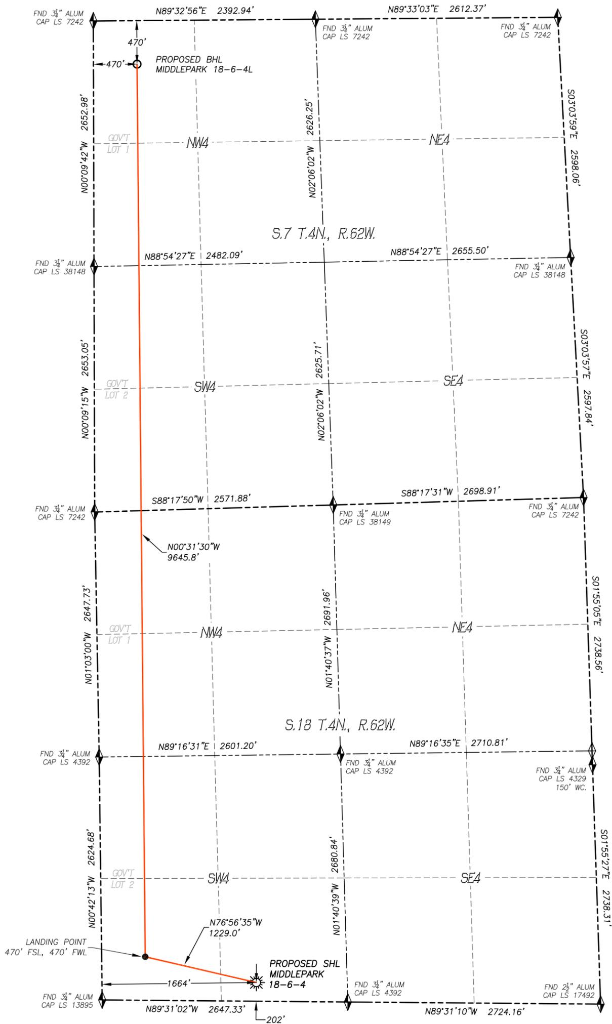
IN ACCORDANCE WITH A REQUEST FROM CONFLUENCE RESOURCES, DALEY LAND SURVEYING, INC. HAS DETERMINED THE SURFACE LOCATION OF THE MIDDLEPARK 18-6-4 WELL TO BE 202 FSL, 1664' FWL, AS MEASURED AT NINETY (90) DEGREES FROM THE SECTION LINES OF SECTION 18, TOWNSHIP 4 NORTH, RANGE 62 WEST, AND THE BOTTOM HOLE LOCATION TO BE 470' FNL, 470' FWL, AS MEASURED AT NINETY (90) DEGREES FROM THE SECTION LINES OF SECTION 7, TOWNSHIP 4 NORTH, RANGE 62 WEST, OF THE 6TH PRINCIPAL MERIDIAN, WELD COUNTY, COLORADO.
