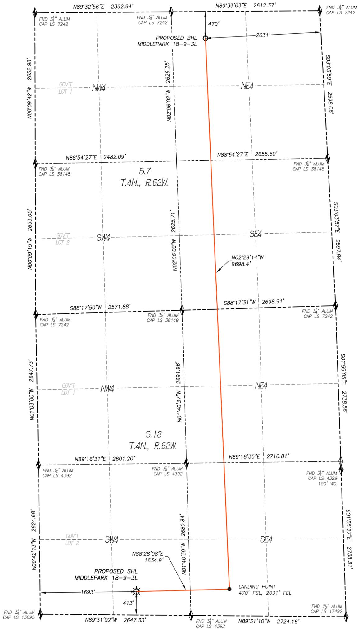
IN ACCORDANCE WITH A REQUEST FROM CONFLUENCE RESOURCES, DALEY LAND SURVEYING, INC. HAS DETERMINED THE SURFACE LOCATION OF THE MIDDLEPARK 18-9-3L WELL TO BE 413' FSL, 1693' FWL, AS MEASURED AT NINETY (90) DEGREES FROM THE SECTION LINES OF SECTION 18, TOWNSHIP 4 NORTH, RANGE 62 WEST, AND THE BOTTOM HOLE LOCATION TO BE 470' FNL, 2031' FEL, AS MEASURED AT NINETY (90) DEGREES FROM THE SECTION LINES OF SECTION 7, TOWNSHIP 4 NORTH, RANGE 62 WEST, OF THE 6TH PRINCIPAL MERIDIAN, WELD COUNTY, COLORADO.
