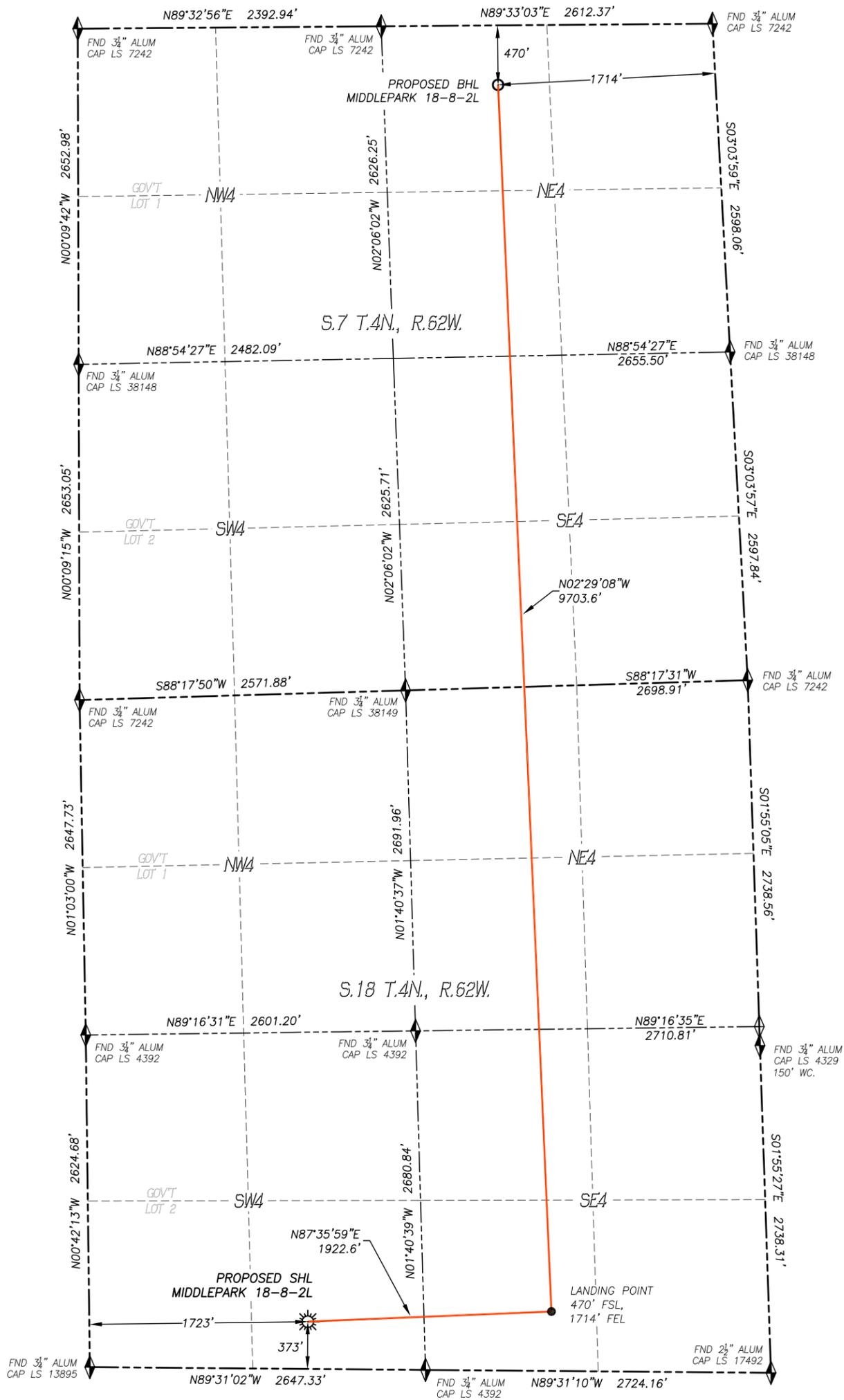
IN ACCORDANCE WITH A REQUEST FROM CONFLUENCE RESOURCES, DALEY LAND SURVEYING, INC. HAS DETERMINED THE SURFACE LOCATION OF THE MIDDLEPARK 18-8-2L WELL TO BE 373' FSL, 1723' FWL, AS MEASURED AT NINETY (90) DEGREES FROM THE SECTION LINES OF SECTION 18, TOWNSHIP 4 NORTH, RANGE 62 WEST, AND THE BOTTOM HOLE LOCATION TO BE 470' FSL, 1714' FEL, AS MEASURED AT NINETY (90) DEGREES FROM THE SECTION LINES OF SECTION 7, TOWNSHIP 4 NORTH, RANGE 62 WEST, OF THE 6TH PRINCIPAL MERIDIAN, WELD COUNTY, COLORADO.
