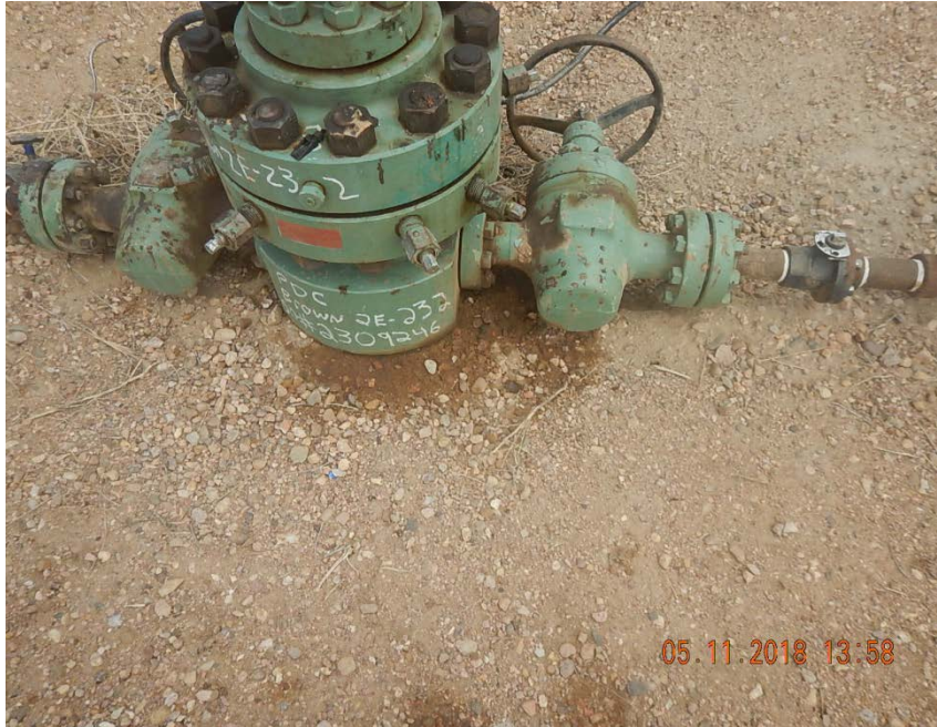
Photo 3: Stained soil at wellhead
