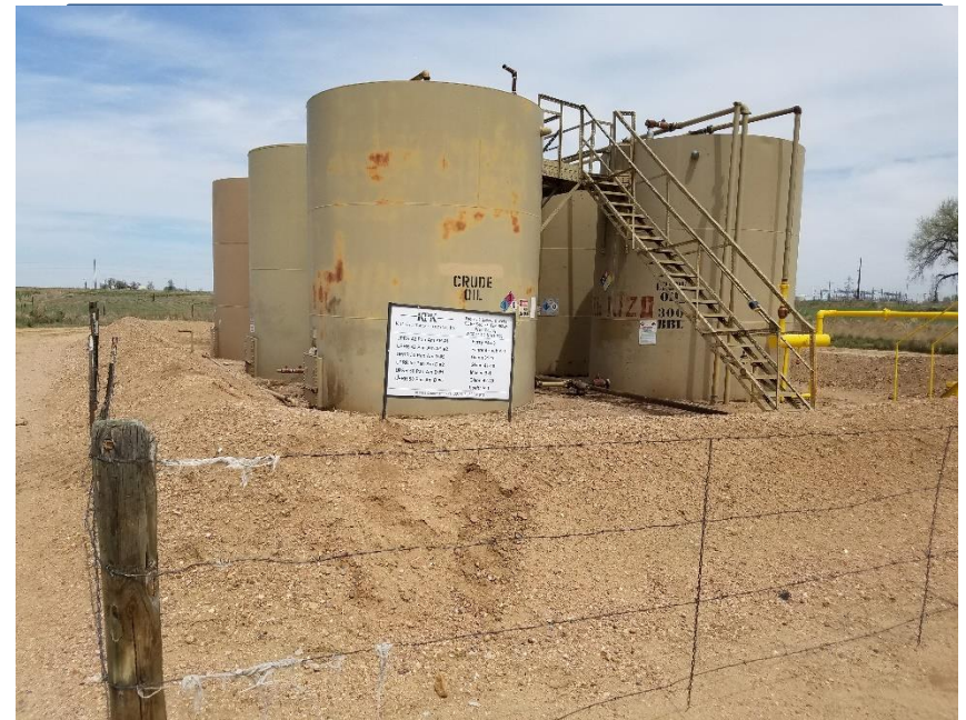
Photo 2. Tank battery
