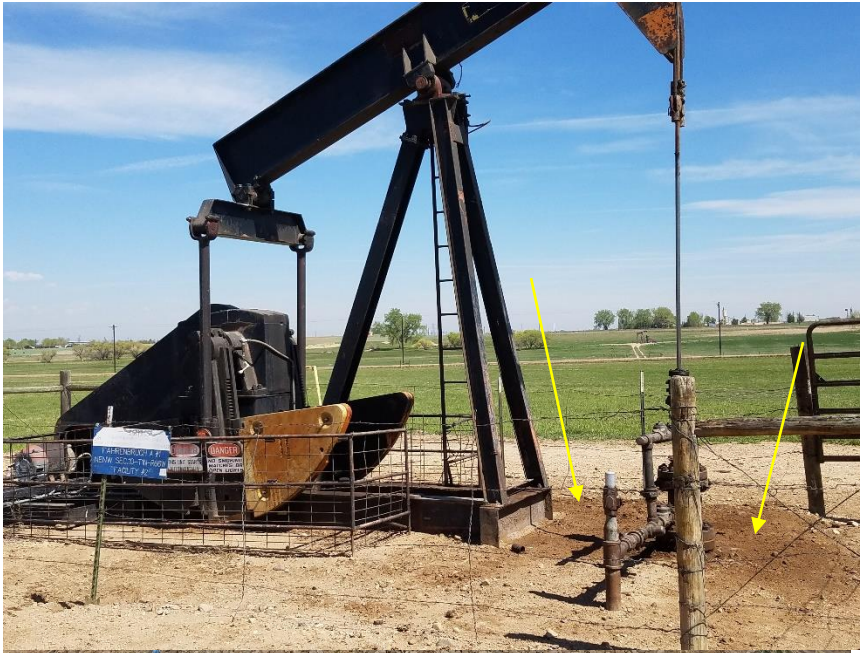
Photo 1. Wellhead, stained soil around wellhead
