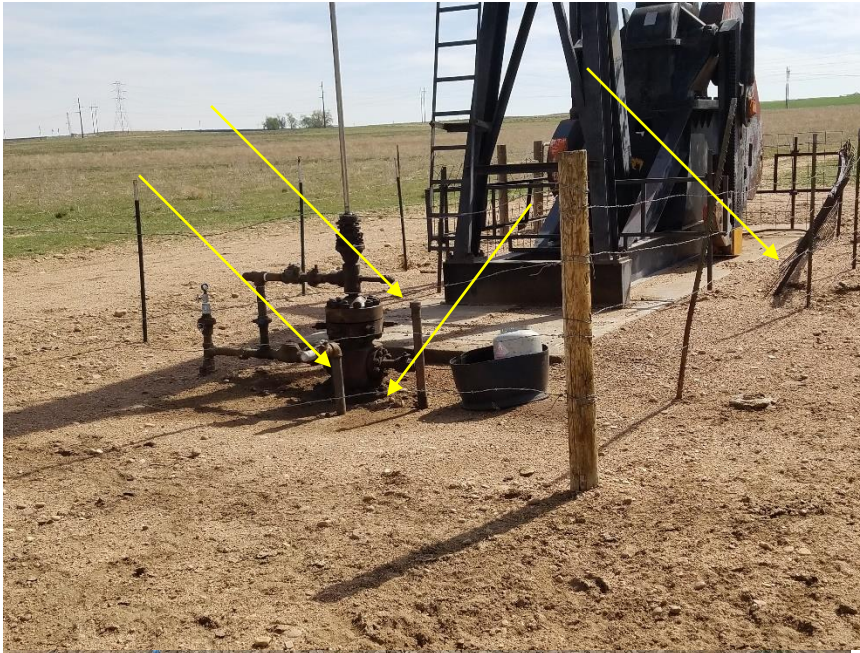
Photo 1. Wellhead, Unmarked risers, stained soil, pumjack guard not attached
