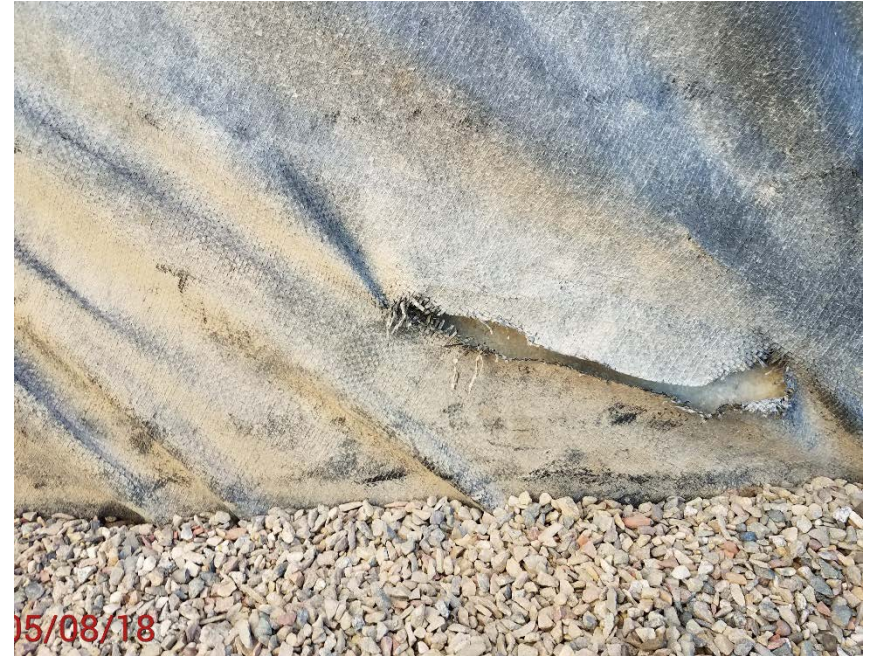
Location photo # 2, Holes in tank battery liner
