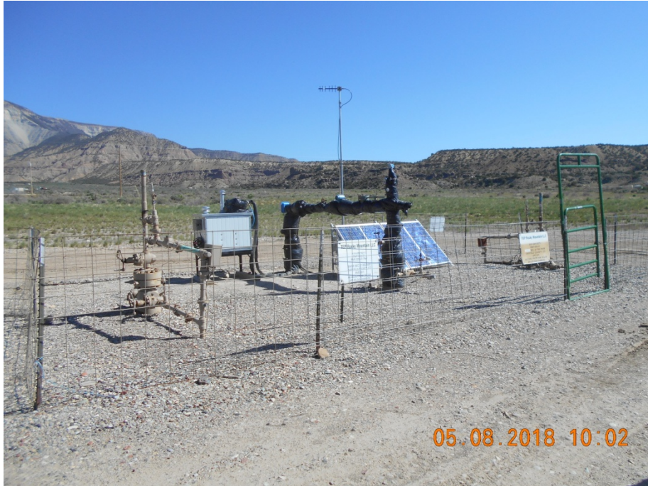
Wellhead with line heater.
