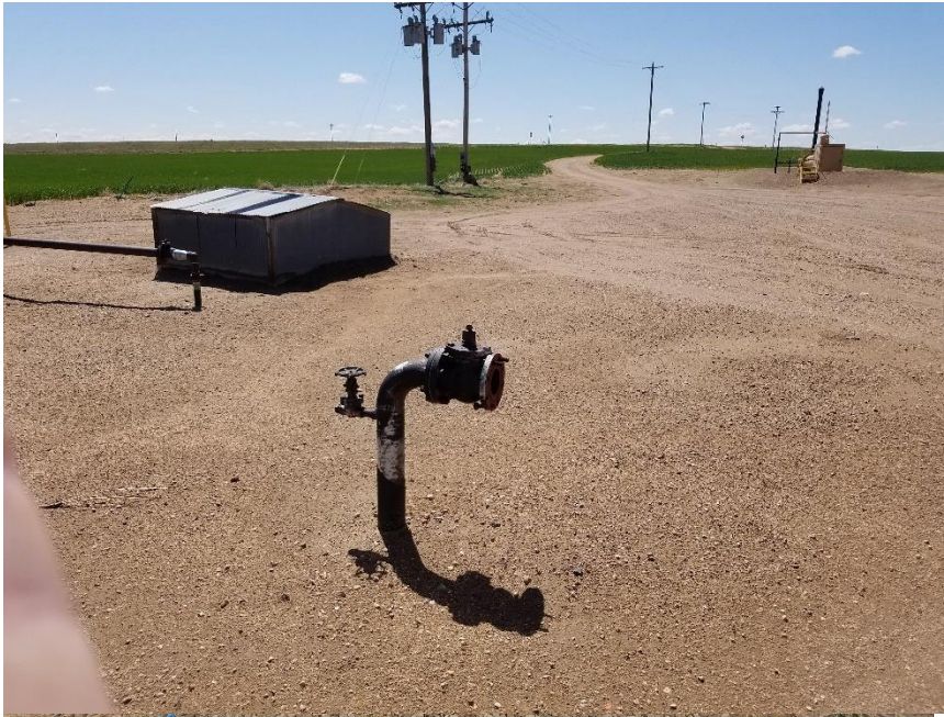
Photo 3. Unmarked riser
