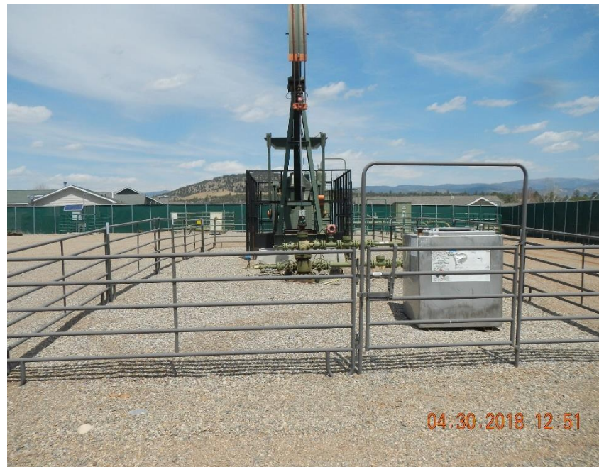
Ludwig #2 well head, pump jack, and chemical injection system.
