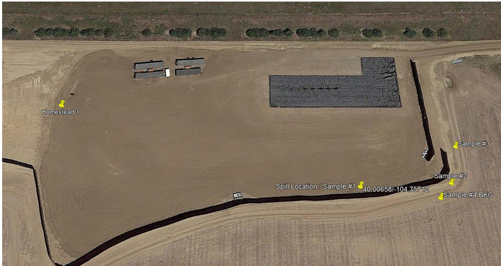
Water from spill ran under sound wall and collected in the stormwater diversion ditch. Water and impacted soil removed via vacuum trucks. Horizontal/Vertical extent of contamination determined with sensory observation and PID. Cleanup confirmation samples were taken on 5/1/18.
