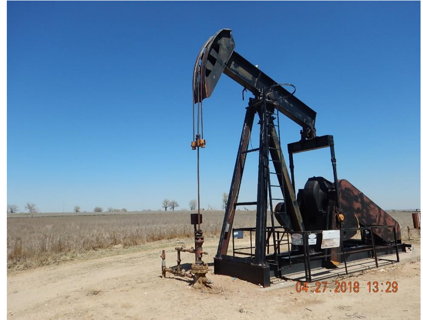
View of pump jack/ wellhead
