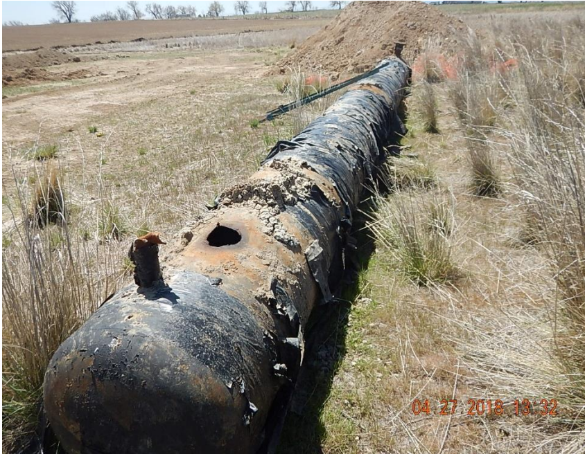
Photo of buried vessel removed from excavation; lacking integrity with obvious corrosion holes
