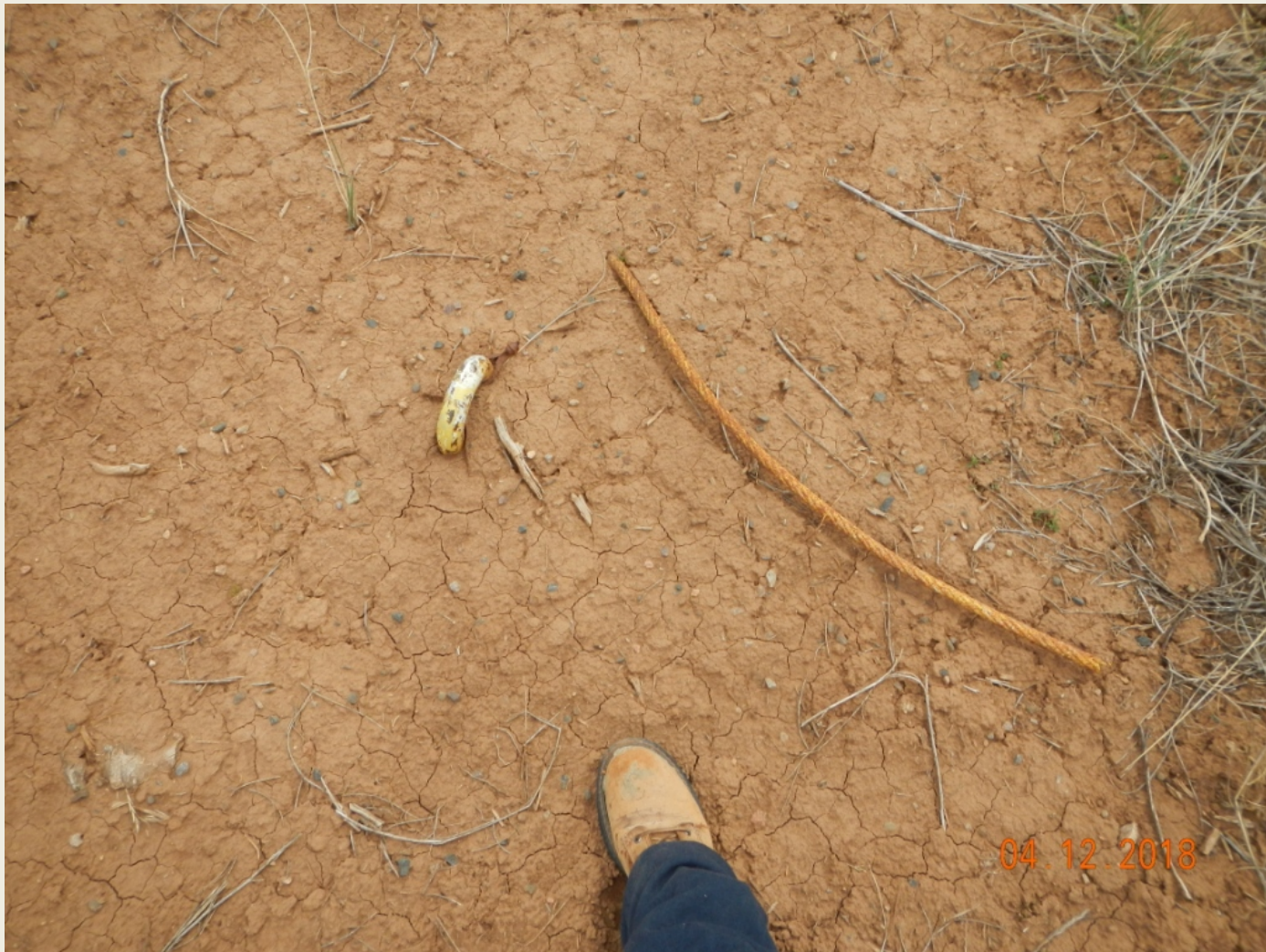
Photo 5. View of another unmarked rig anchor within the project area.
