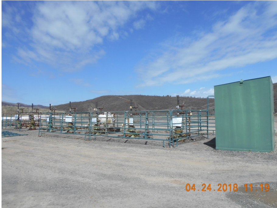
Wellheads with signs. Injection wellhead inside housing
