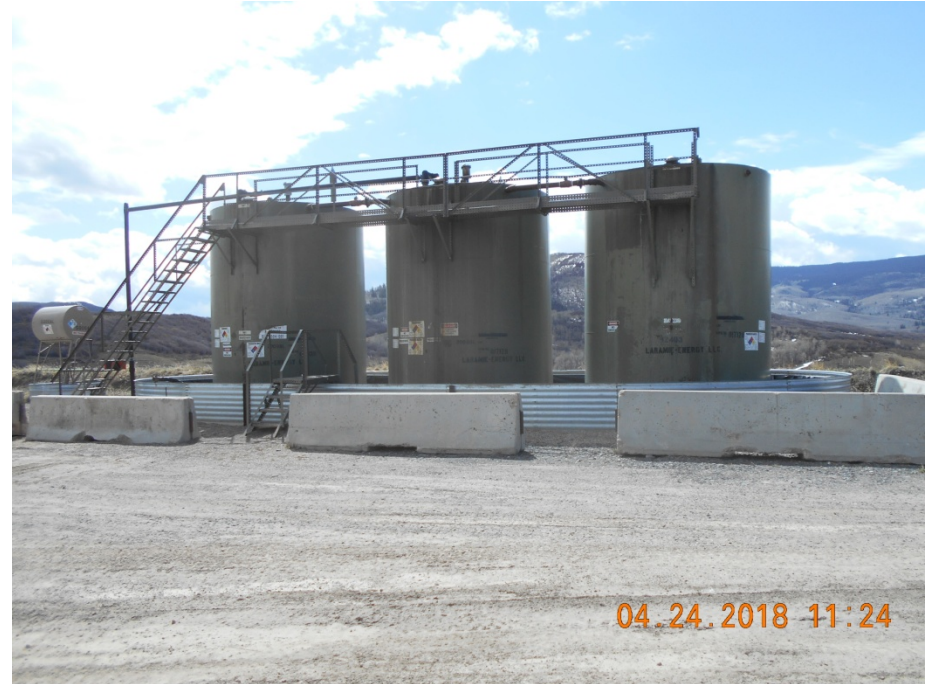
Condensate Tank battery
