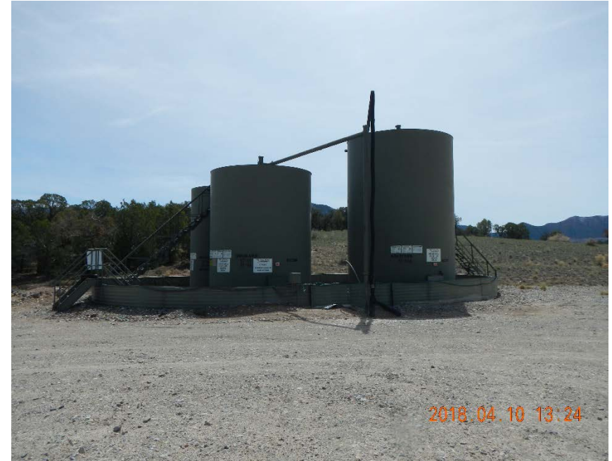
One 500 bbls tank and two 300 bbls tank. A pinhole leak was discovered on the 500 bbls tank. The tank will be removed.
