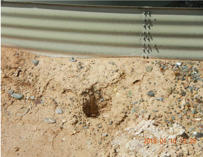
Caerus investigated the perimeter of the tank battery. Borehole(s) on the north side filled with water during hydrostatic test.
