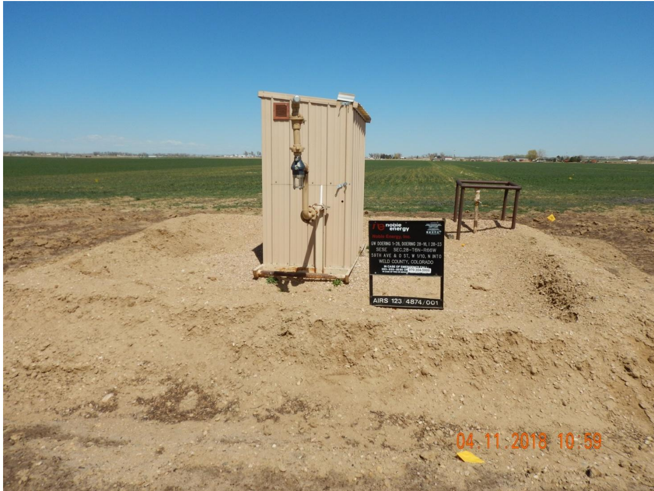
Photo 1. Photo taken from the battery location, facing North. Operator has failed to remove equipment within three months of plugging (meter house and riser).
