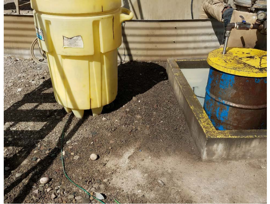
Photo #4 Stained soil around filter pot
