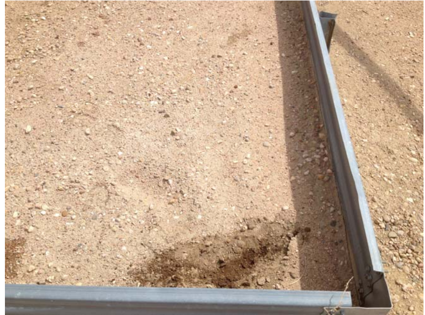
Photo 4 – Impacted soil beneath clean gravel at southwest corner heater treater secondary containment
