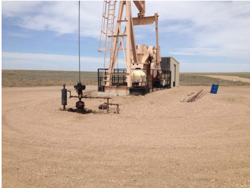
Photo 7 – Wellhead area with unused rods and lube oil drum with no secondary containment.
