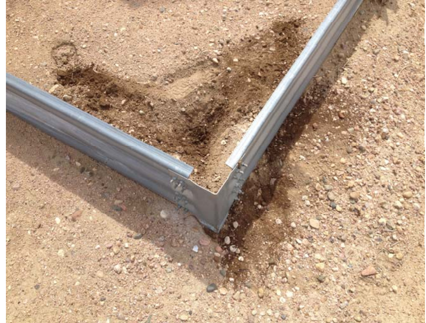
Photo 2 – Impacted soil beneath clean gravel at northwest corner of heater treater secondary containment
