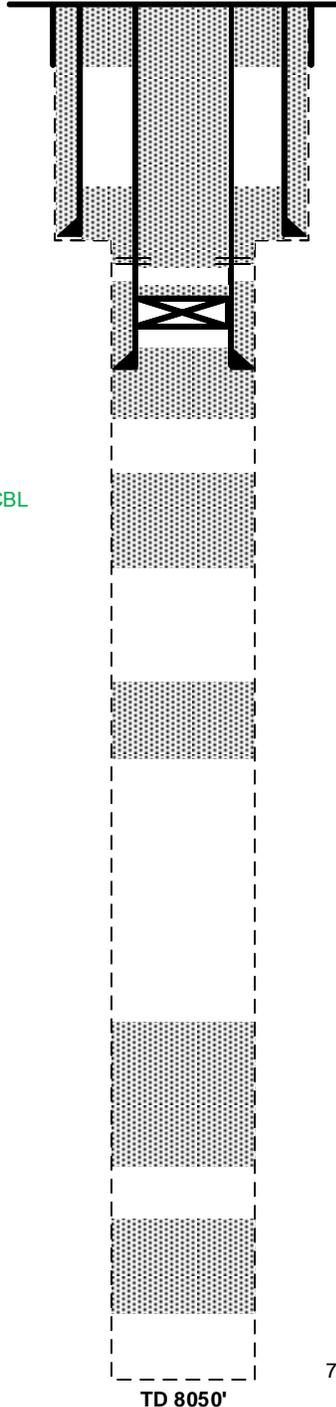
Washed down 8-5/8" x 7" annulus to 53'. Pumped annular fill with 5 sx Class G from 53' to surface.
