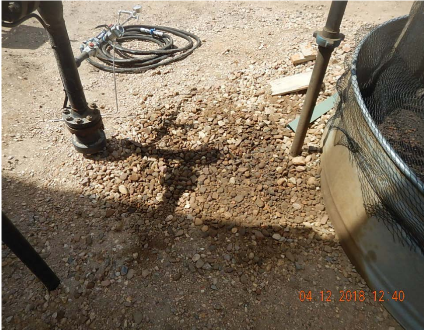
Photo 13: Stained soil at engine oil container.
