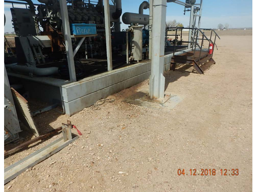
Photo 4: Stained soil at compressor
