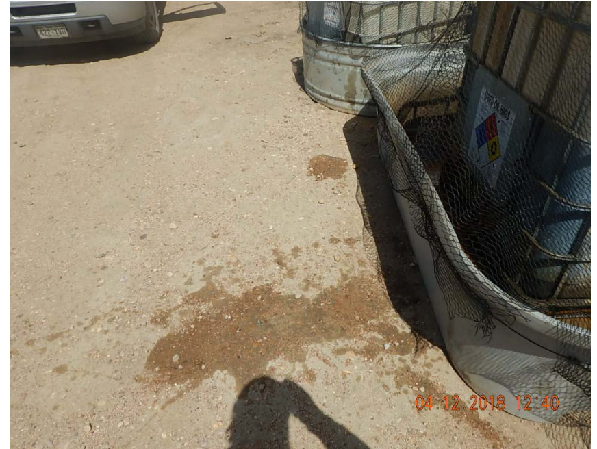
Photo 14: Stained soil at used engine oil container.
