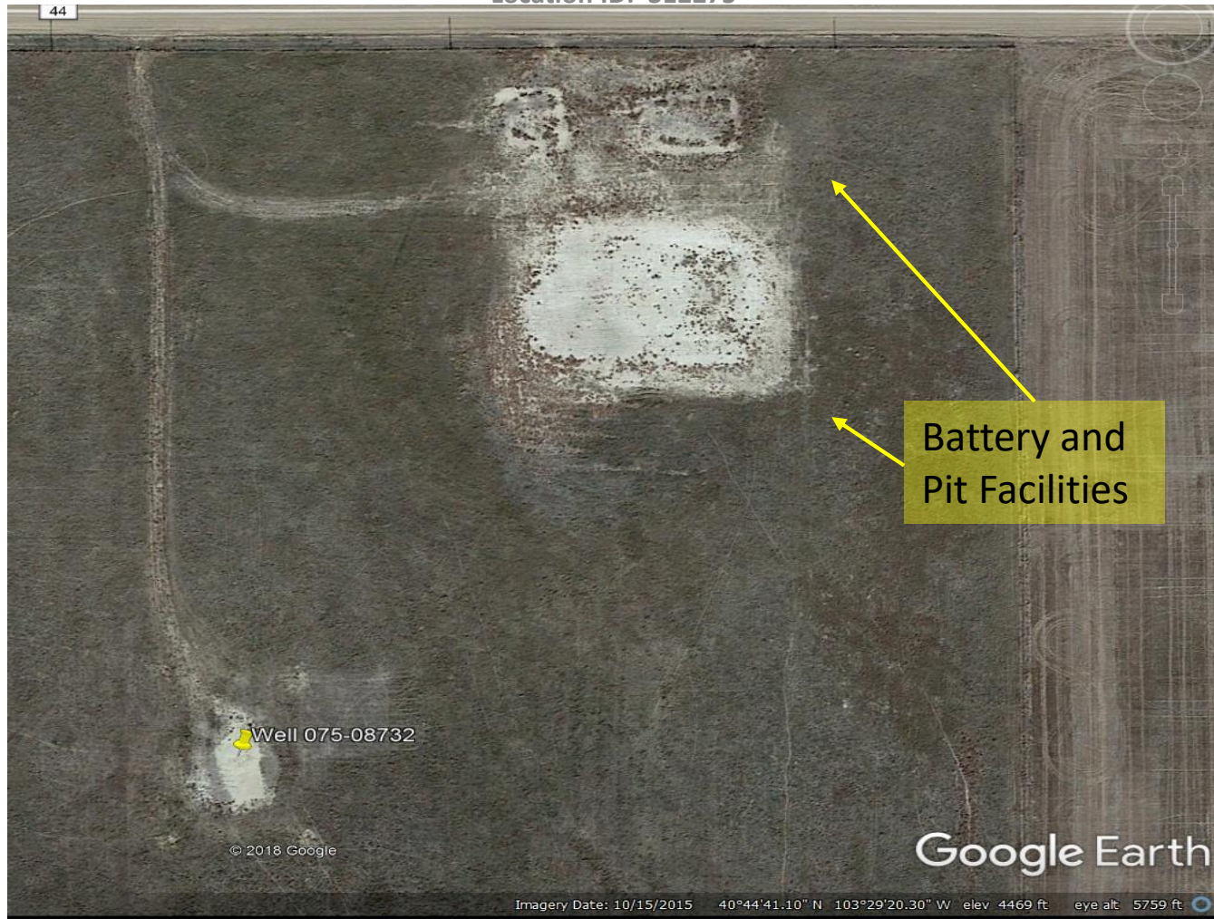
Photo 19: Most current available aerial imagery (10/15/2015). Photo shows areas of the well, battery and pit facilities after plugging and abandonment of the location. Photo also shows large areas of the location that appear to be predominantly bare and exposed soil.
