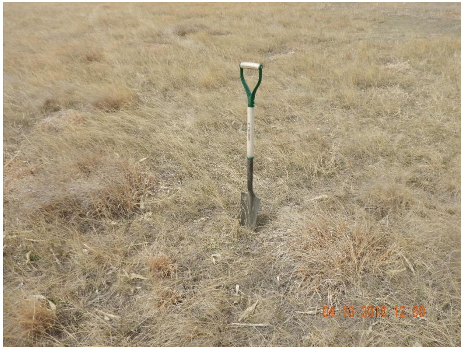
Photo 5: Photo taken from the adjacent reference area. Photo shows inspector tested the reference area compare/contrast to the disturbance for compaction concerns. Photo shows inspector was able to penetrate the top 8 inches of soil with relative ease.
