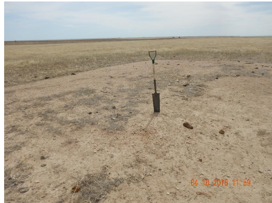
Photo 4: Photo taken from the well location, facing north. Photo shows inspector tested the location for compaction concerns; inspector was only able to penetrate the first few inches of the disturbance area. It does not appear as though compaction alleviation has been conducted in accordance to 1004.a
