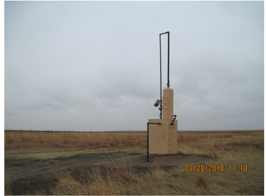
2. Meter shed with vertical gas separator
