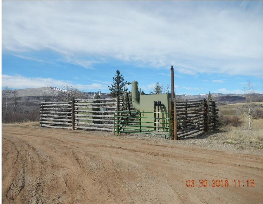
Meter run and separator for Falcon Seaboard 12 #1.
