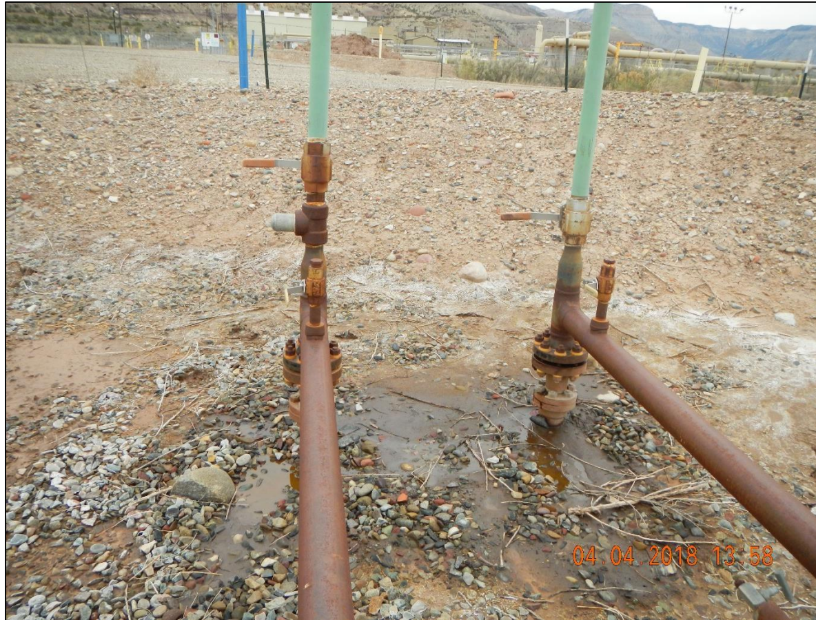
Leak and spill behind separators.
