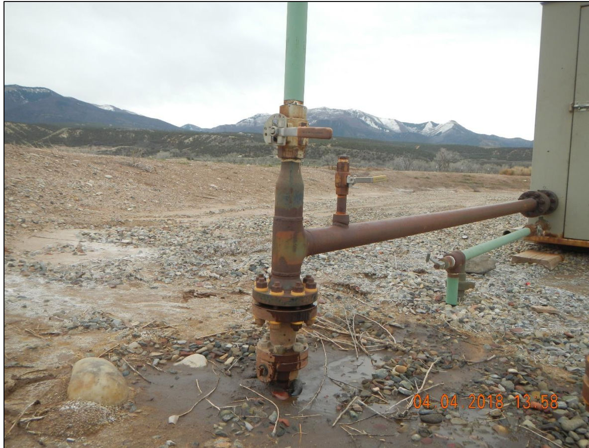
Leaking at flange.
