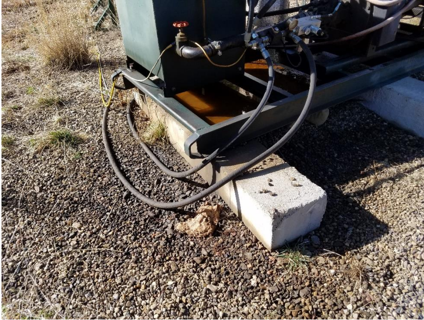
Photo 1. Stained soil around prime mover
