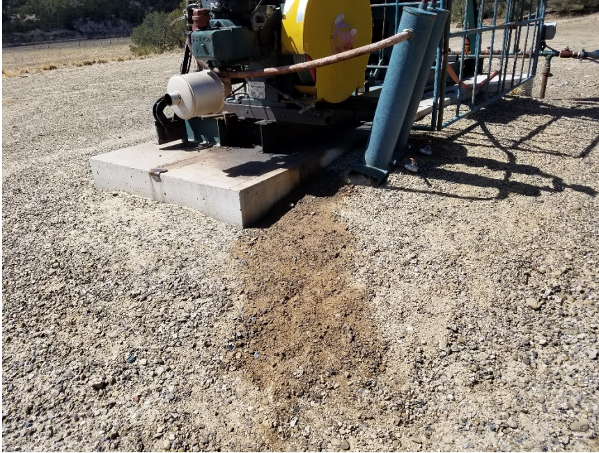
Photo 1. Stained soil around prime mover
