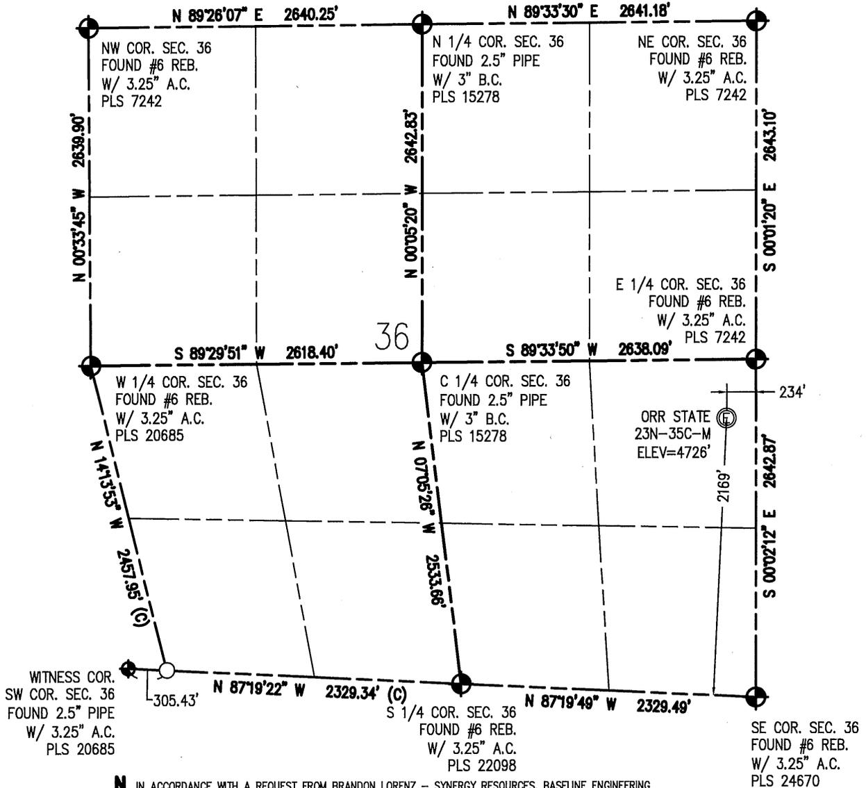
IN ACCORDANCE WITH A REQUEST FROM BRANDON LORENZ - SYNERGY RESOURCES, BASELINE ENGINEERING CORP. HAS DETERMINED THE LOCATION OF THE ORR STATE 23N-35C-M TO BE 2169' FSL AND 234' FEL, AS MEASURED AT NINETY (90) DEGREES FROM THE SECTION LINE OF SECTION 36, TOWNSHIP 6 NORTH, RANGE 67 WEST, 6TH PRINCIPAL MERIDIAN, WELD COUNTY, COLORADO.
