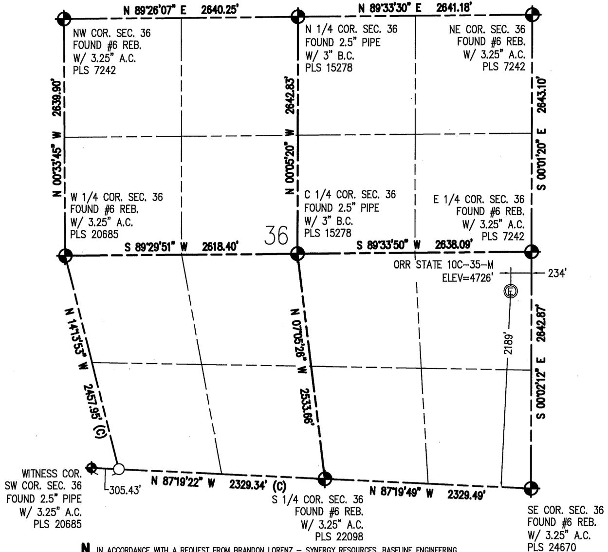
IN ACCORDANCE WITH A REQUEST FROM BRANDON LORENZ - SYNERGY RESOURCES, BASELINE ENGINEERING CORP. HAS DETERMINED THE LOCATION OF THE ORR STATE 10C-35-M TO BE 2189' FSL AND 234' FEL, AS MEASURED AT NINETY (90) DEGREES FROM THE SECTION LINE OF SECTION 36, TOWNSHIP 6 NORTH, RANGE 67 WEST, 6TH PRINCIPAL MERIDIAN, WELD COUNTY, COLORADO.
