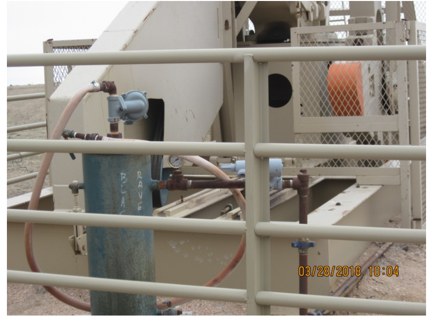
2. Prime mover has been removed
