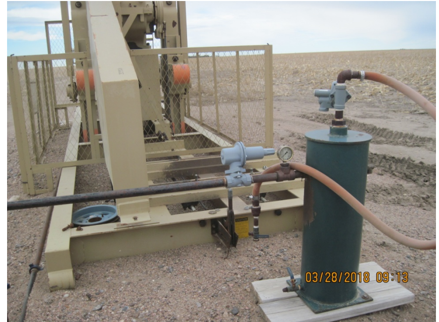
2. Prime mover has been removed
