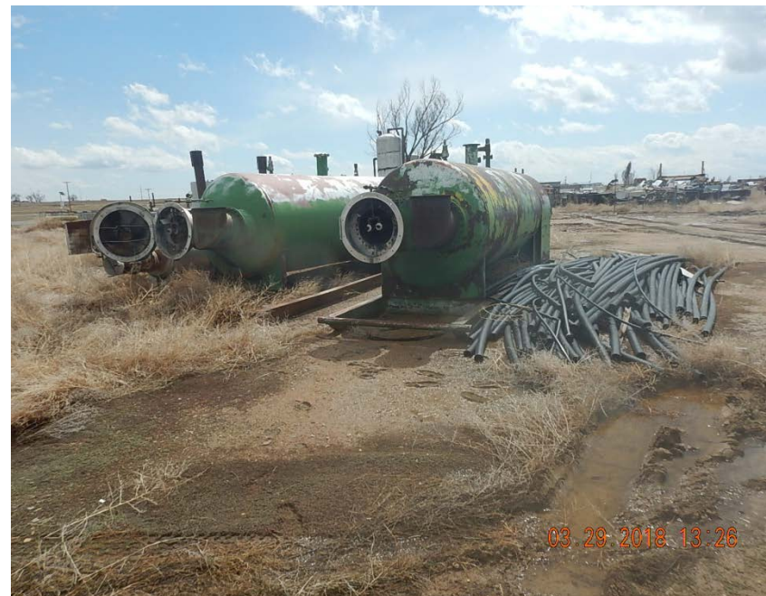
Photo 12: Unused separators, rods in center of location (E of compressor)
