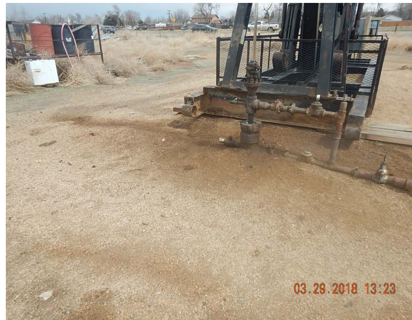
Photo 8: Stained soil, contaminant migration at Dacono 1
