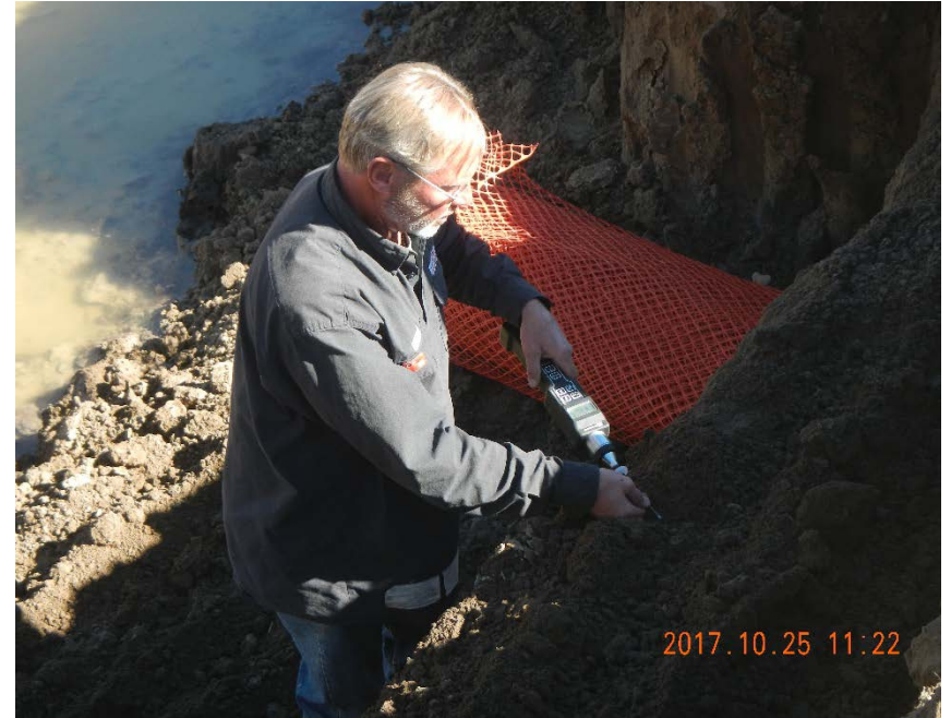
Field screening walls of the excavation
