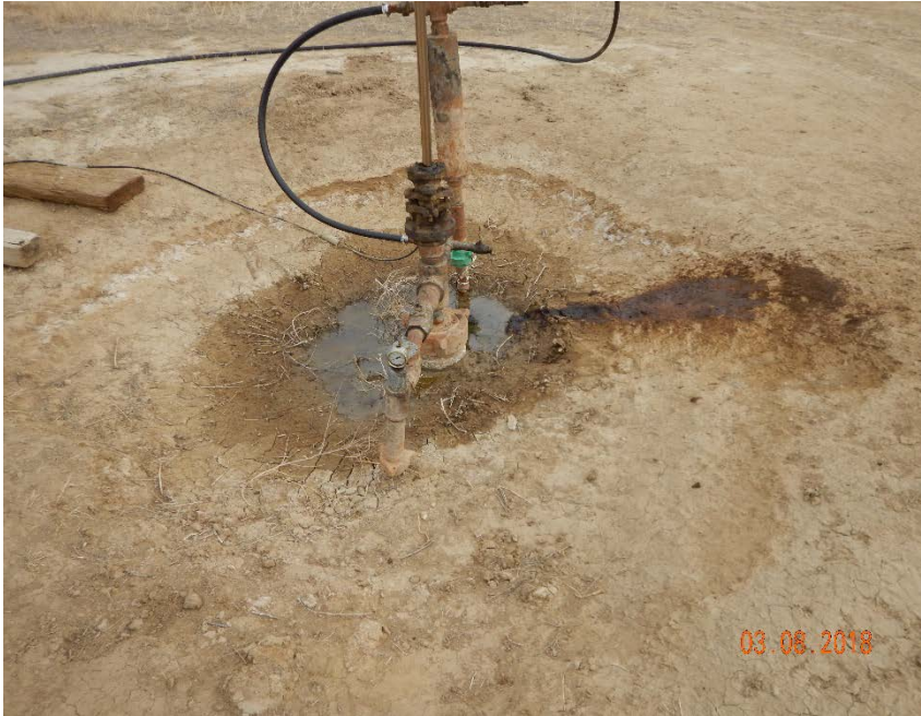
Photo #3 – View of oily waste spray, puddle of water, and evaporite accumulation at wellhead from west.
