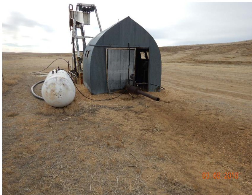
Photo #5 – Accumulation of blow-through motor oil extending from prime mover exhaust.
