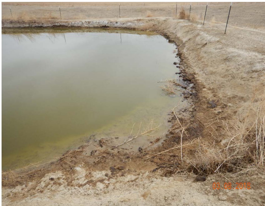
Photo #17 – Oil-stained soil remaining inside of south pit berm.
