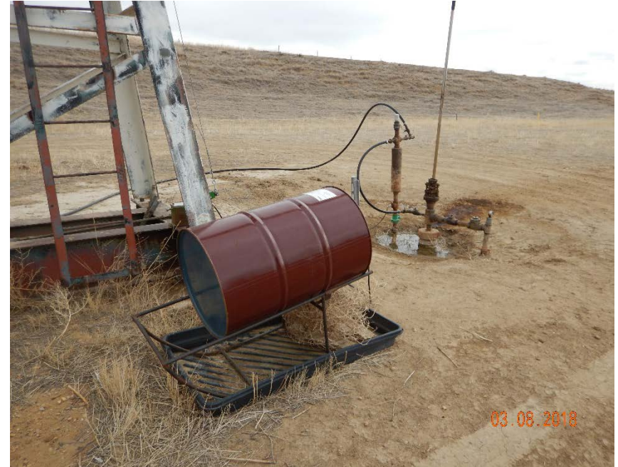
Photo #2 – View of secondary containment device and wellhead from NW.
