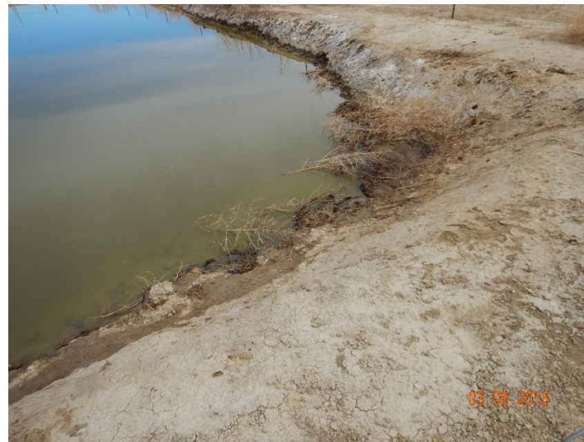
Photo #18 – Accumulation of oily waste inside of SE corner of produced water pit.
