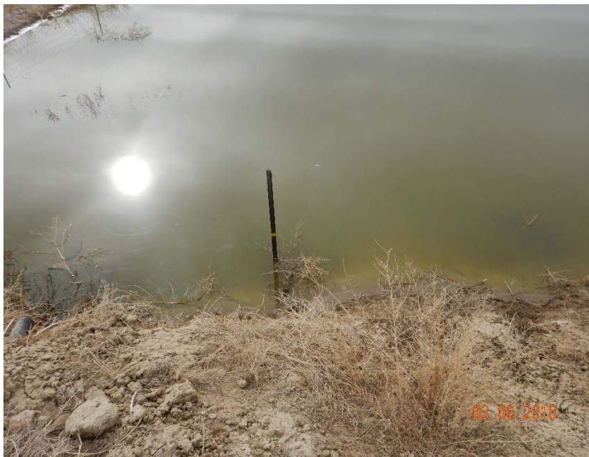
Photo #15 – T-post has been installed at NE corner of produced water pit as a means of monitoring freeboard.
