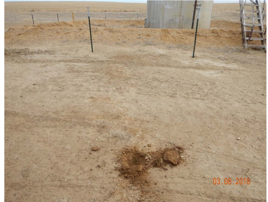
Photo #24 – Photo from inspection date (March 8, 2018) depicting oil-stained soil that remains in area west of existing crude oil AST berm.
