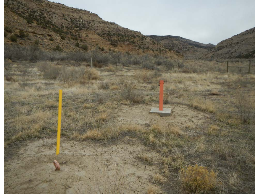
Single remaining monitoring well in former source area
