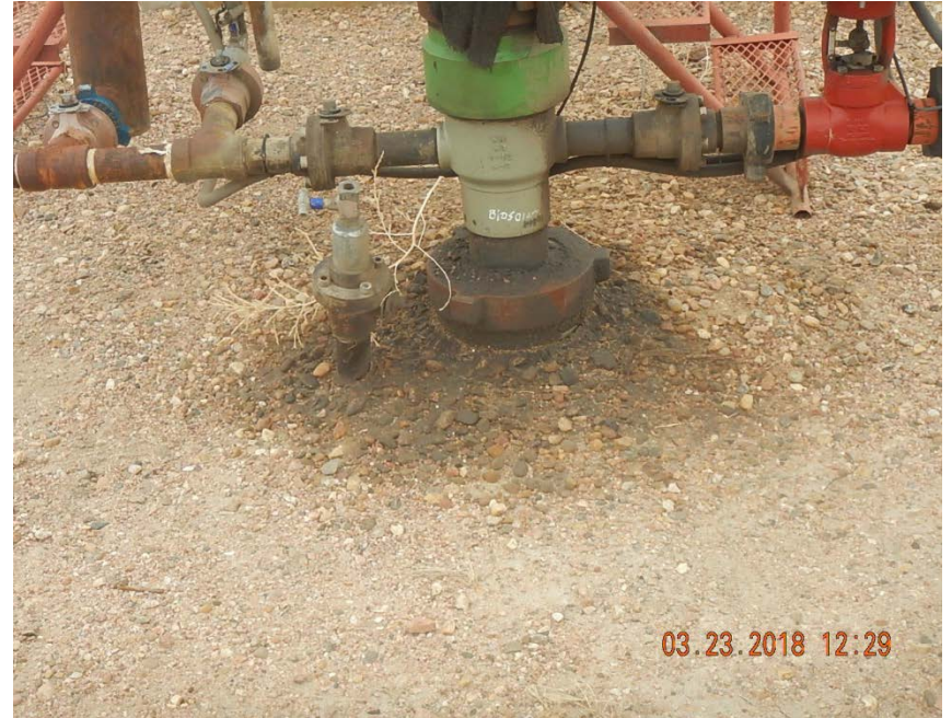
Photo 2: Stained soil at wellhead
