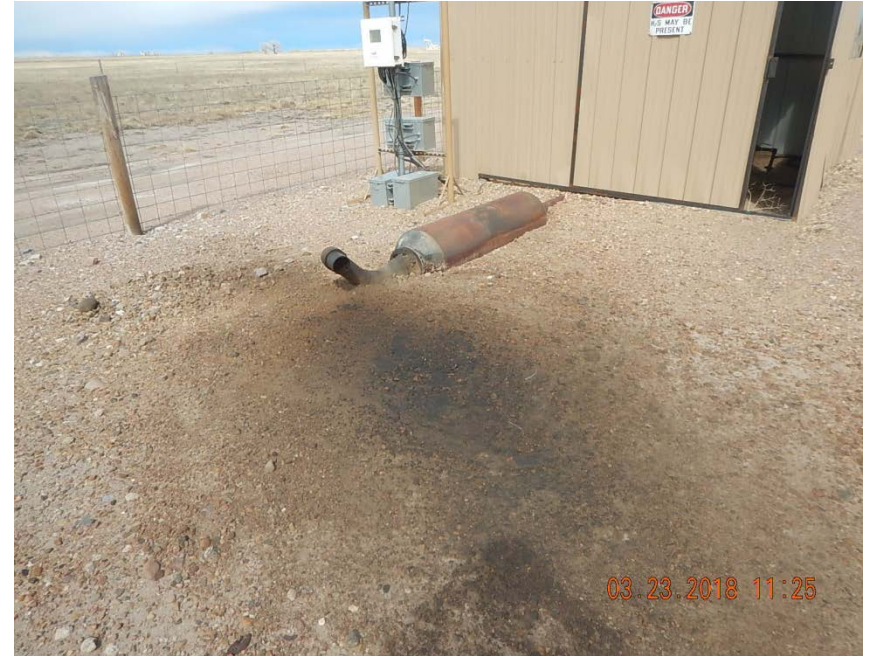
Photo 2: Stained soil at exhaust
