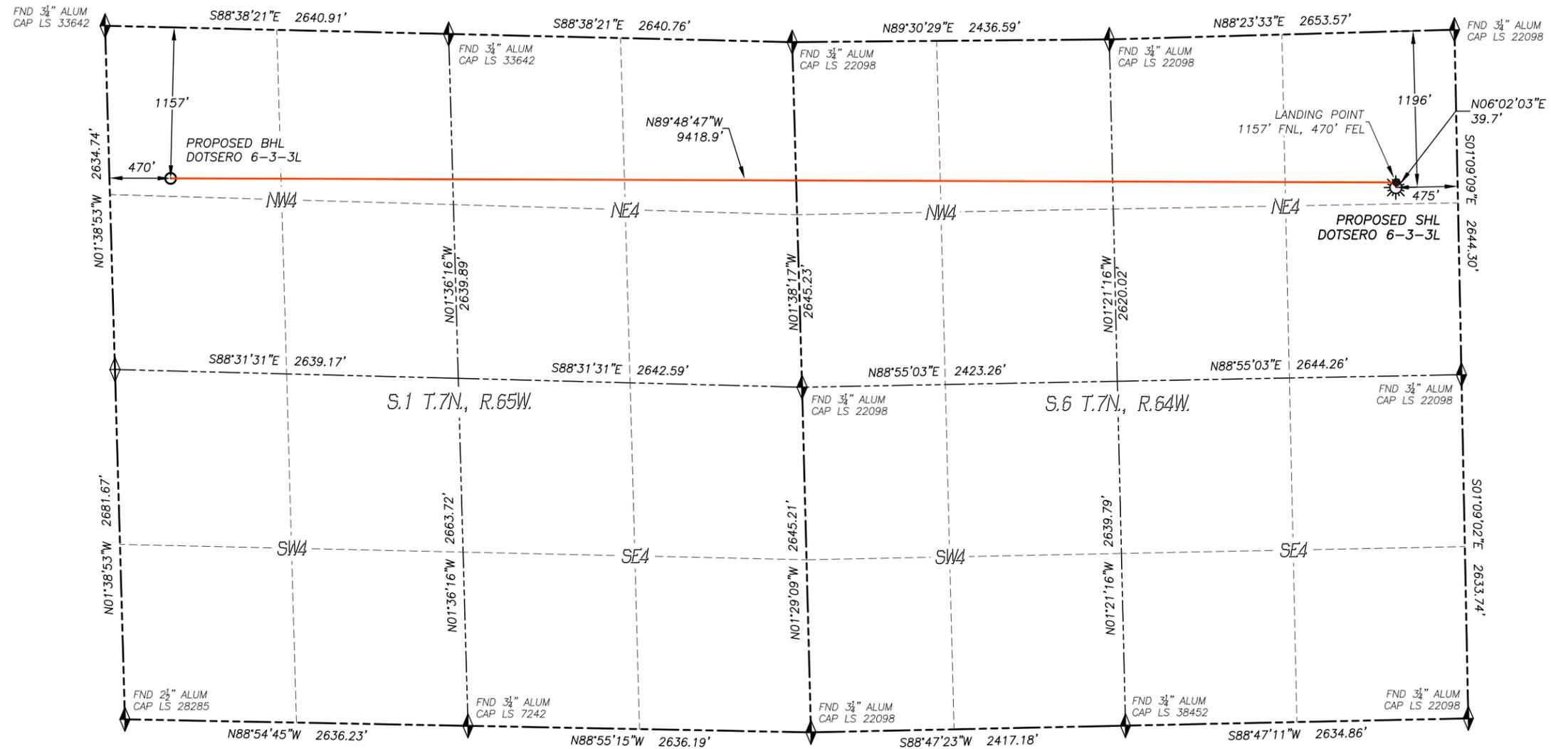
IN ACCORDANCE WITH A REQUEST FROM CONFLUENCE RESOURCES, DALEY LAND SURVEYING, INC. HAS DETERMINED THE SURFACE LOCATION OF THE DOTSERO 6-3-3L WELL TO BE 1196' FNL, 475' FEL, AS MEASURED AT NINETY (90) DEGREES FROM THE SECTION LINES OF SECTION 6, TOWNSHIP 7 NORTH, RANGE 64 WEST, AND THE BOTTOM HOLE LOCATION TO BE 1157' FNL, 470' FWL, AS MEASURED AT NINETY (90) DEGREES FROM THE SECTION LINES OF SECTION 1, TOWNSHIP 7 NORTH, RANGE 65 WEST, OF THE 6TH PRINCIPAL MERIDIAN, WELD COUNTY, COLORADO.
