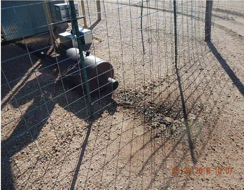
Photo 5: Stained soil at engine exhaust.
