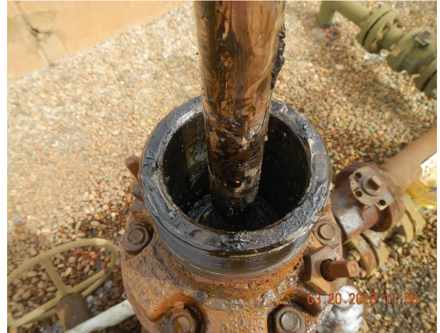
Worn out packing rings were allowing gas and fluids to escape.
